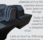
ARMORLUG® ULTRA is the first patented drive lug with three fabric layers embedded in Easily handles today's biggest, most powerful tractors and
