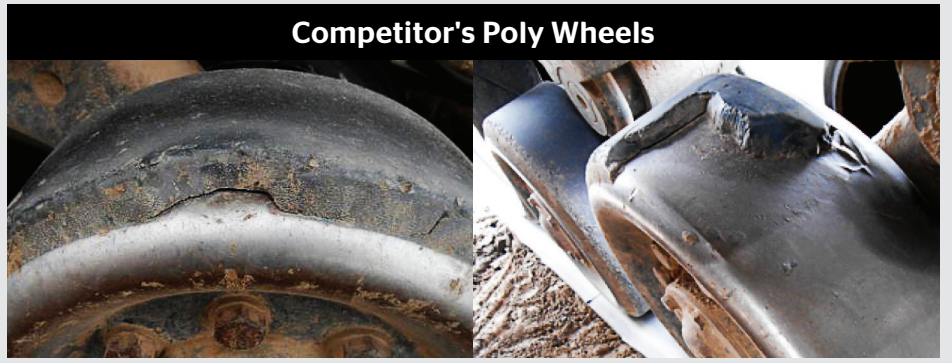
Major damage to outer surface and significant separation from the metal hubs.
