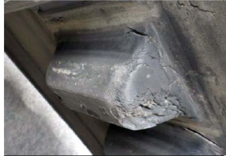
Typical Drive Lug Mid-Life Wear
